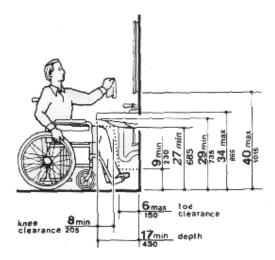
Mirrors - Mirrors located above lavatories or countertops shall be installed with the bottom edge of the reflecting surface 40 inches (1015 mm) maximum above the finish floor or ground. Mirrors not located above lavatories or countertops shall be installed with the bottom edge of the reflecting surface 35 inches (890 mm) maximum above the finish floor or ground.
